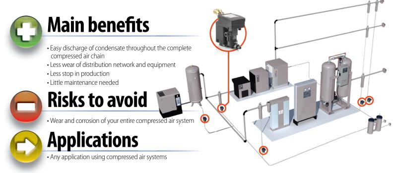
The new LD range functions using a system called capacitive condensate discharge. Compared to the traditional timer condensate discharge system, it has several advantages.
